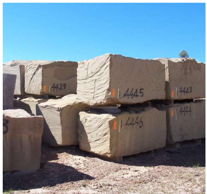
Yellowblock (Pyrmont) quarry stones from the Department of Commerce's stockpile
